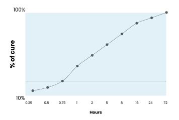
The graph shows the rate of cure for a M10
